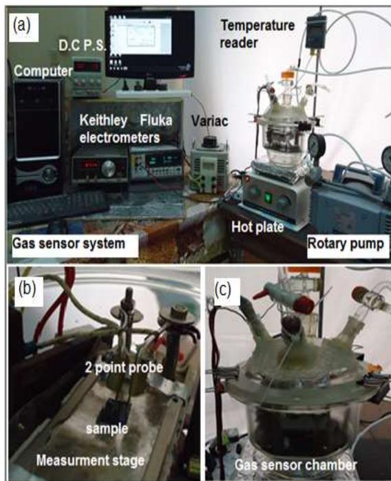
**Figure 10: Photograph of the homemade gas sensor system; (a) complete setup; (b) measurement stage; and (c) glass reaction chamber/ (UOT).**
