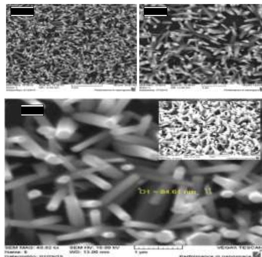
**Figure 4: SEM images of ZnO NRs/SiO<sub>2</sub>/Si (111), hydrothermally synthesized at 85 °C for 2h, and with 30 mM seed layer concentration (Inset image is tilted 30°)**
