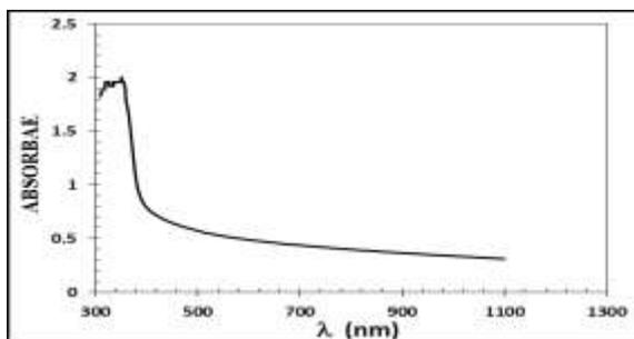
Figure 6: Absorbance spectrum of the annealed ZnO NRs film
