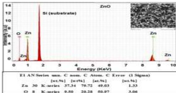
Figure 5: EDS spectrum of annealed ZnO NRs film with the Zn and O elements composition
