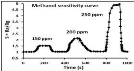
**Figure 12: Sensor sensitivity versus time at various methanol concentrations.**
