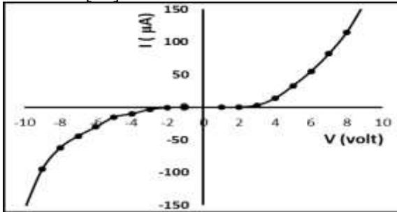
**Figure 9: I-V characteristics for ZnO NRs /SiO<sub>2</sub>/Si (111), hydrothermally synthesized at seed layer concentration of 30 mM.**
