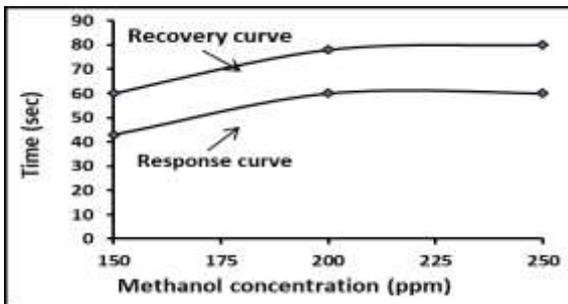
**Figure 14: Response and recovery time curves versus various methanol concentrations.**
