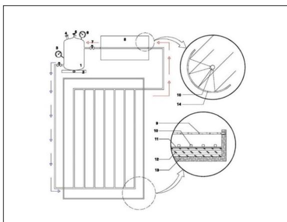
**Figure 2: Schematic diagram of the solar water heater partition showing its components and flow. (1) Feed tank. (2) Heater electric. (3) Temperature gage. (4) Groundwater feed. (5) Water vapor outlet. (6) Pressure gage. (7) Valve. (8) Parabolic trough solar concentrator. (9) Glass sheet. (10) Copper pipe (11) Aluminum plate. (12) Insulation 50 mm. (13) wood panel. (14) Chrome plate.**
