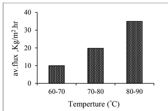
Figure 3: Effect of feed temperature on water flux
