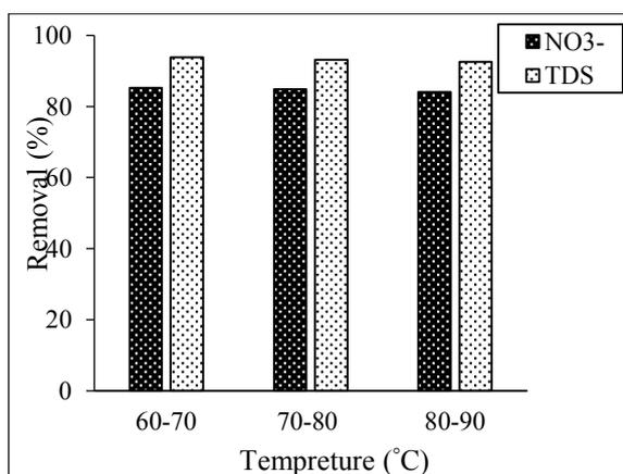
Figure 6: Effect of feed temperature on NO<sub>3</sub>- and TDS removal efficiency
