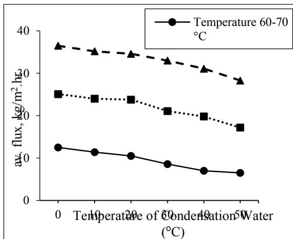
Figure 5: Effect of condensate temperature on water flux
