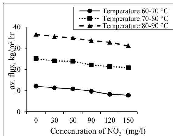
Figure 4: Effect of nitrate concentration on water flux
