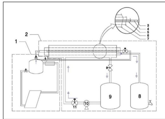
**Figure 1(a):** schematic diagram for the experimental setup. (1) Solar water heater partition (2) Nitrate removal partition. (3) Perforated polyethylene pipe. (4) Holes 5mm at 25mm. (5) Jute rope. (6) Aluminum pipe. (7) Plastic cover. (8) Cold water tank. (9) Distillate water tank. (10) Pump. (11) Valve.
