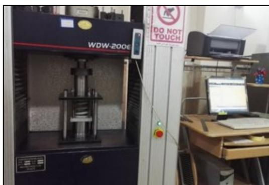
Figure 7: RPSMF die mounted to the computerized testing machine
